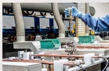
This is the aim of our plating department at Socapex: with perfectly controlled bath processes, they modify and/or add a thin layer of metal on the connectors to make them more efficient and resistant! For example, we propose a plating of Nickel, Cadmium or Black Zinc Nickel on Aluminium to protect the connector!
