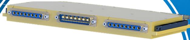
**PSD28V16CEC-X is a 16-channel power distribution unit, designed for land vehicle applications. It distributes 28VDC through overload and short-circuit protected switches. The PSD28V16CEC -X supports CAN and RS-485 communication to control, configure and get the status of the device.**
