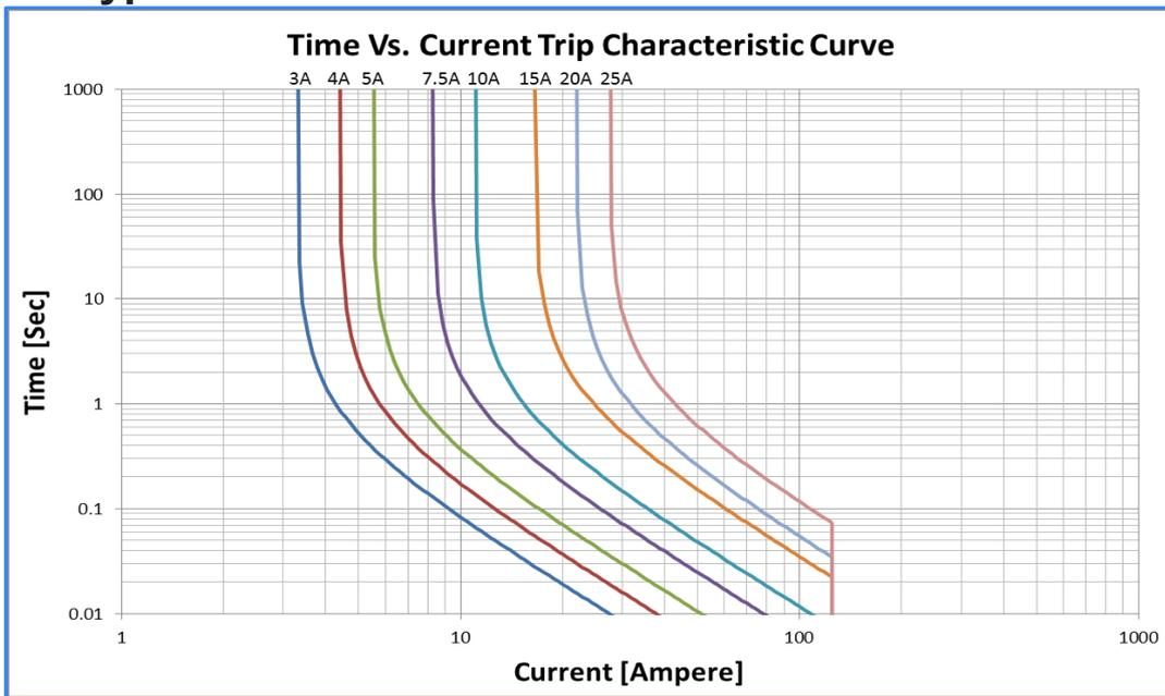
Figure 1 - Time vs. Current Overload Trip
