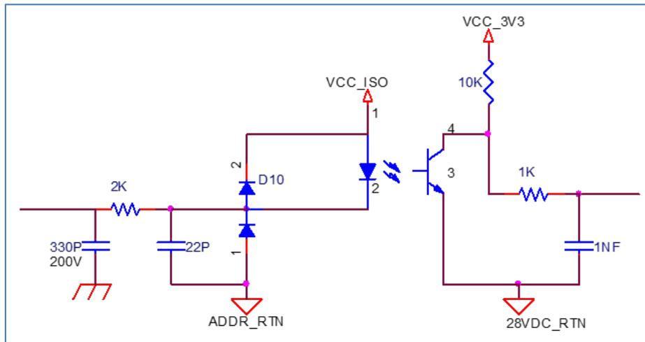
Figure 4 – Address input interface
