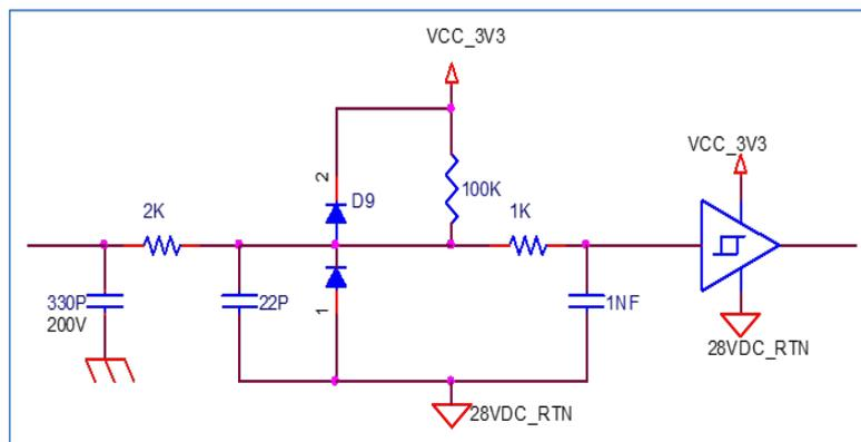
Figure 3 – Discrete input interface
