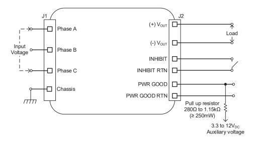
**Note:** PWR GOOD pull-up resistor and auxiliary voltage shown in this diagram are typical values. The system designer must select the actual values such that no damage can occur to the internal components of the power supply – *consult factory for more information*.
