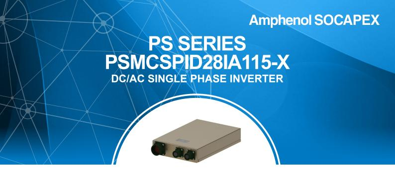
The PSMCSPID28IA115-X is a baseplate-mount, conduction-cooled, DC/AC inverter designed for rugged airborne applications that convert electrical power in aircraft from nominal 28 volts power to single-phase alternating current power 115VAC or 230VAC at 50/60/400 Hz. The product is design to meet MIL-STD requirements (specified herein).
