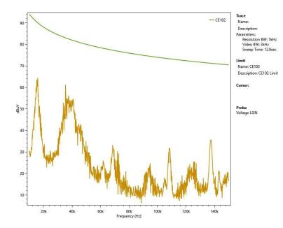
**CE102 MIL-STD-461F Conducted Emission, 10 kHz -150 kHz** Return (nominal input voltage, full load)
