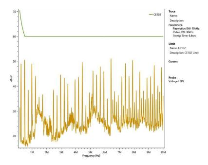
CE102 MIL-STD-461F Conducted Emission, 150 kHz -10 MHz Line (nominal input voltage, full load)
