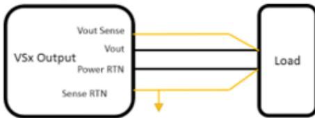
Figure 3: PSVA6USTPU115P1100-0 Sense Lines
