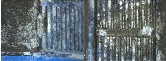
Figure 12: Corrosions areas onto knurling of the locking nut of connectors
