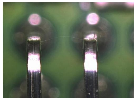
Figure 4: Illustration of a Tin whisker bridging two conductors.
