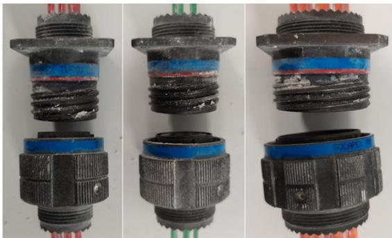
Figure 13: Series III SnZn plated connectors size 13, 15 and 21
