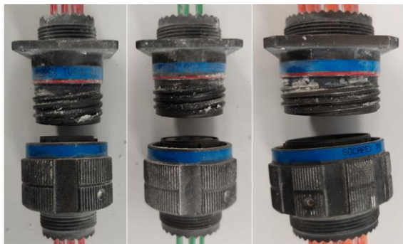
Figure 13: Series III SnZn plated connectors size 13, 15 and 21 (from left to right) after Gr 11 tests before cleaning (after dust test) Amphenol Socapex.
