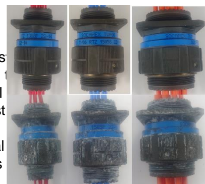
Figure 11: SnZn plated connectors size 13, 15, 21. Before (up) and after (down) Neutral Salt Spray test. Amphenol Socapex.
