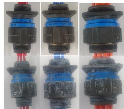
Figure 11: SnZn plated connectors size 13, 15, 21. Before (up) and after (down) Neutral Salt Spray test. **Amphenol Socapex.**
