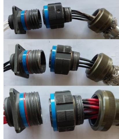
Figure 15: SnZn plated connectors size 13, 15 and 21 (from up to down) after Gr 14 tests
