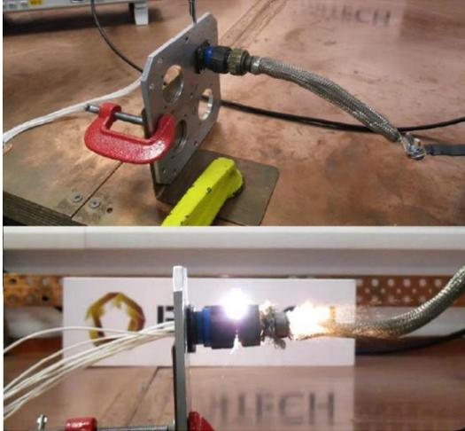
Figure 14. Indirect lightning test setup (up) and testing (down)
