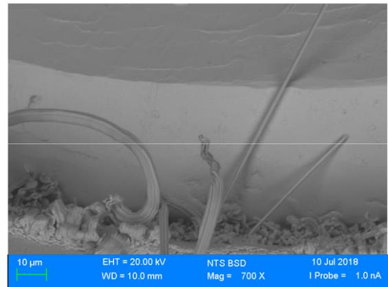
Figure 5: SEM picture of a starting site of Tin whiskers by compressive forces.
