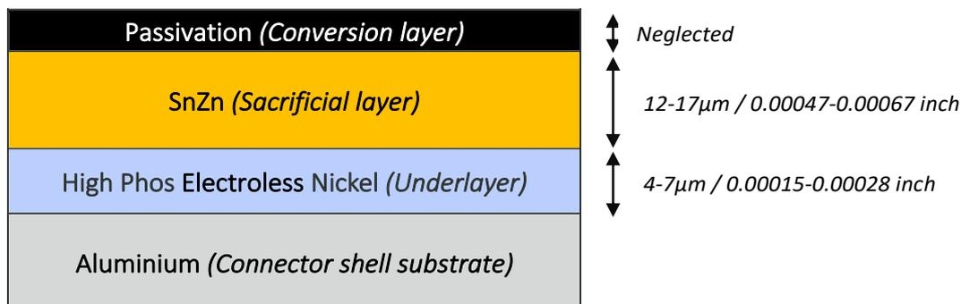
Figure 3: Illustration of a SnZn architecture over High Phosphorus Electroless Nickel and Aluminum.
