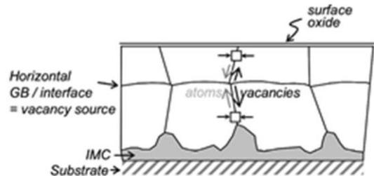
Figure 7: Schematic showing how horizontal boundaries act as vacancy sources (or atom sinks), absorbing the atom flux flowing up vertical boundaries. [6]
