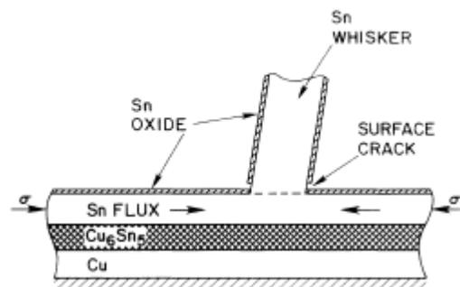
Figure 8: Illustration of the cross section of the Cu-Sn IMC and a whisker that grows from an oxide barrier breakage, growing by the migration of Tin atoms [8]
