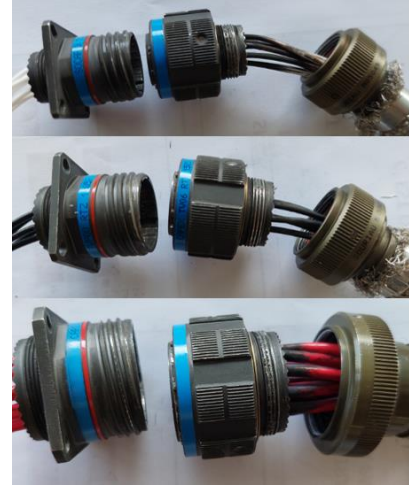
Figure 15: SnZn plated connectors size 13, 15 and 21 (from up to down) after Gr 14 tests Amphenol Socapex.
