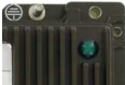
Power LED indicator
