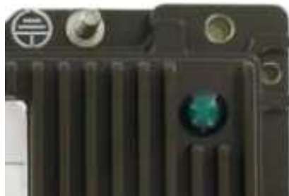
Power LED indicator
