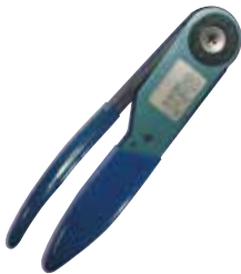
MANUAL CRIMPING PLIERS M22520/1-01
