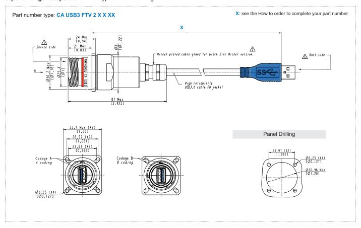
Jam nut receptacle - Shell type 7 - Hexagonal nut mounting
